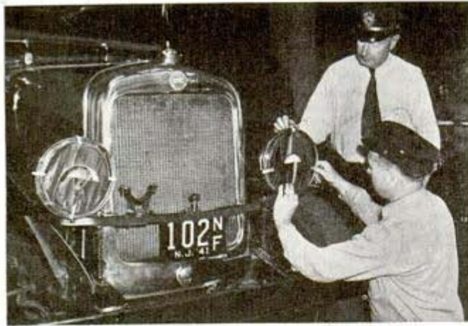
Placing masks over headlights of a fire truck in preparation for a run during a blackout test. Traffic in the blackout is dangerous and nonessential cars must be kept off streets
